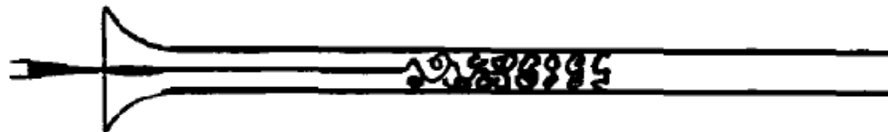
(c) Turbulent flow (observed by electric spark)
