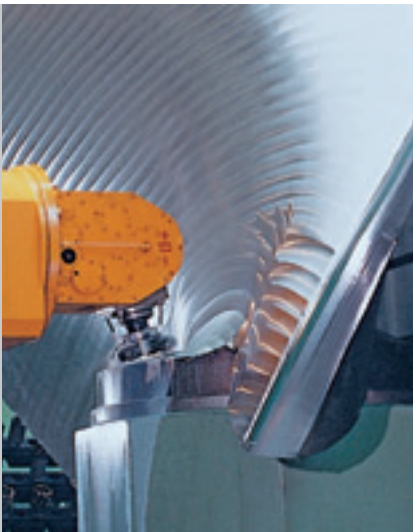
Milling of a Kaplan blade on the 5-axis-CNC-machining center
