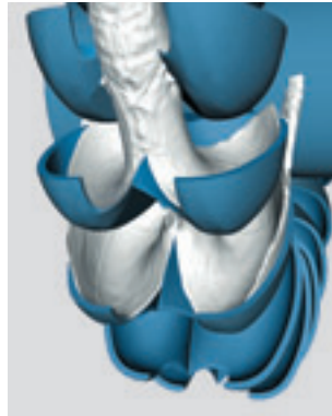
Simulated flow through Pelton runner
