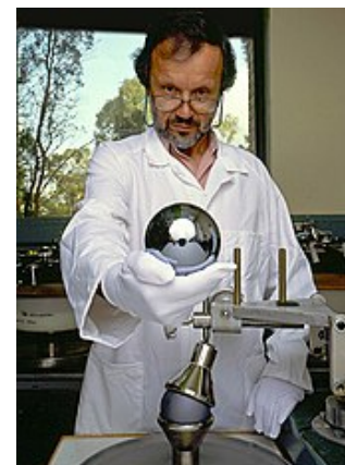
A near-perfect sphere of ultra-pure silicon – part of the Avogadro project, an International Avogadro Coordination project to determine the Avogadro number. [40]
