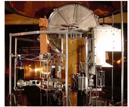
A Kibble balance, which is being used to measure the Planck constant in terms of the international prototype kilogram. [40]
