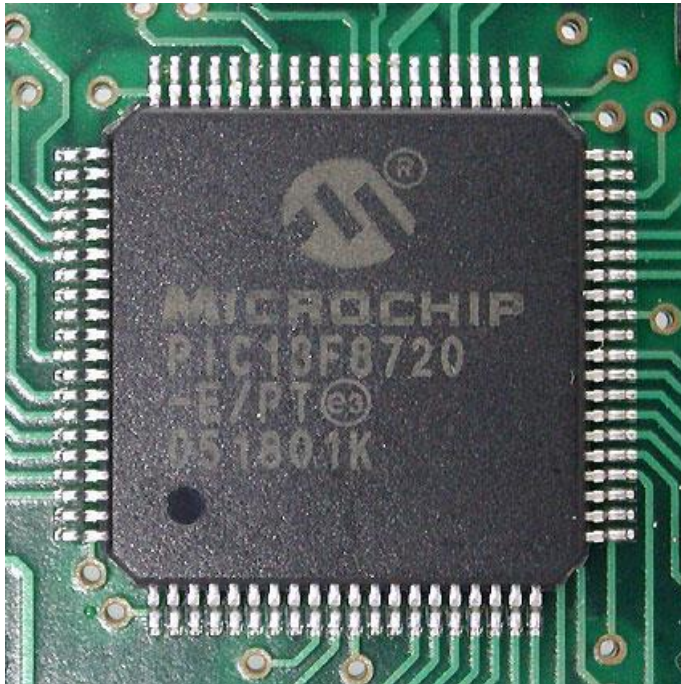
Microcontrollore PIC 18F8720 in contenitore 80-pin TQFP .
