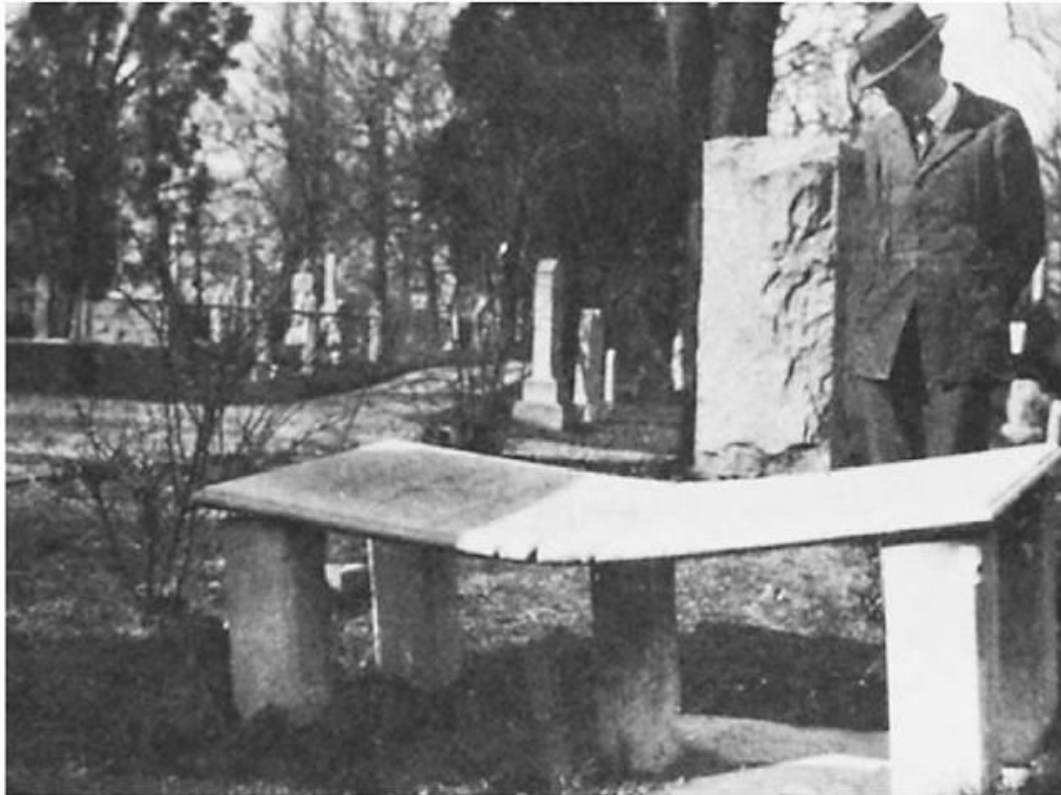
FIGURE 9.38 Sharply dressed man with deformed marble bench that plastically sagged and locally fractured under the influence of gravity [and users].
