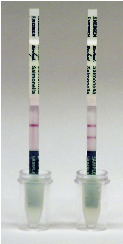
Fig. 1. Commercially available lateral flow immunoassay (Reveal 2.0, Neogen Corporation; see Ref. 38 ) used for the detection of S enterica in equine fecal and environmental samples (see Refs. 17,39,57 ). Test strip on the left indicates a negative test (only the control line is visible); the test strip on the right indicates a positive test (the test line [ lower line ] is as intense in color as the control line [ the top line ]).
