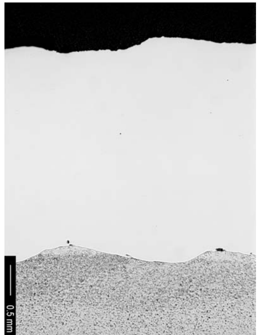
Fig. 12.20 Optical micrograph showing the cross section of the alloy 625 overlay of an overlaid waterwall sample (Fig. 12.19) obtained from a RDF boiler (Lawrence, MA) after 16 years of service. Micrograph also shows the fusion boundary and substrate carbon steel. Courtesy of Welding Services Inc.
