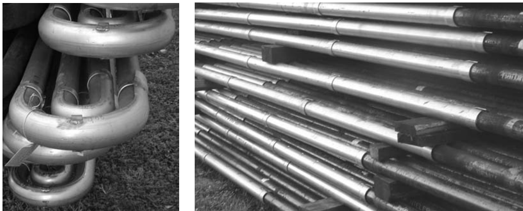
Fig. 12.30 Carbon steel superheater tubes protected by metallic tube shields awaiting installation at one WTE plant.
