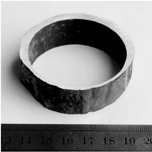
Fig. 12.24 Carbon steel (SA178A) superheater tube after 11 months of service in a mass-burning unit. The superheated steam temperature and pressure were 400 °C (750 °F) and 4.5 MPa (625 psig), respectively. Courtesy of Welding Services Inc.
