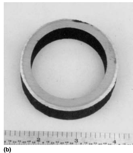
Fig. 12.29 Alloys 72 overlay superheater tube (a) and alloy C276 overlay superheater tube (b) after 7200 operating hours (10 months) in a RDF unit. The windward side of the tube, where the flue gas impinged upon the tube surface was the top side of the tube cross section as shown in the figure. The tube cross section was polished and etched with nital to reveal alloy 625 overlay (white portion of the metal) which was not etched by nital. Courtesy of Welding Services Inc.
