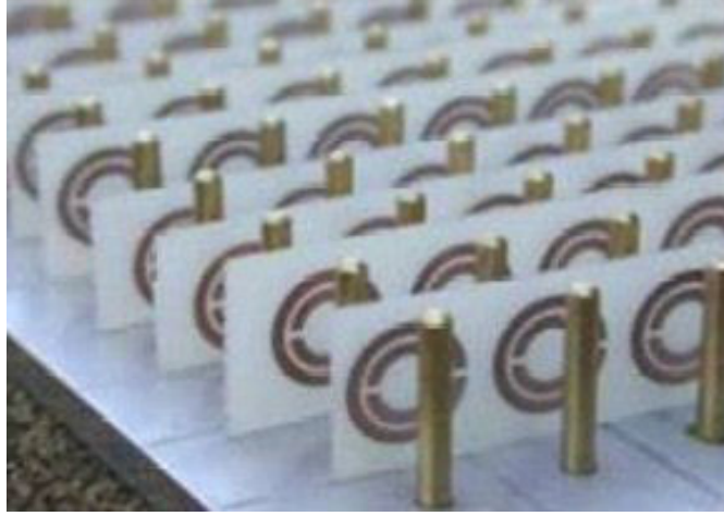
Figure 10: The realization of a DNG material at microwave frequencies with an array of wires and SRRs.
