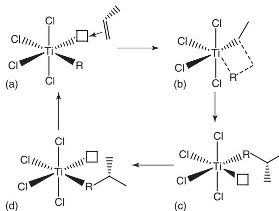
Figure 5.9 The Cossee–Arlman mechanism a) Olefin coordination, b) Olefin concerted insertion, c) Insertion step, d) Chain migration.
