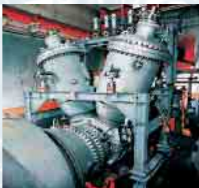
13 Gas turbine test bed - view of gas turbine THM 1304 with DLN combustion chamber
