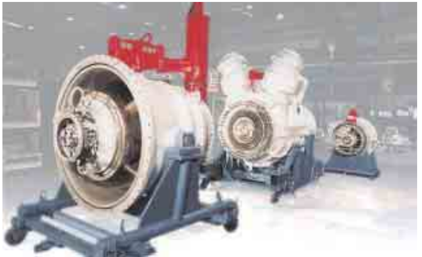
1 Modular design with power turbine, gas generator and air inlet casing (from left to right)
