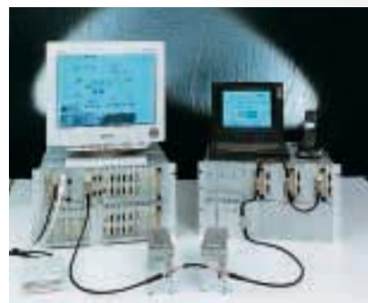
5 "turbolog® DSP" control and protection system
