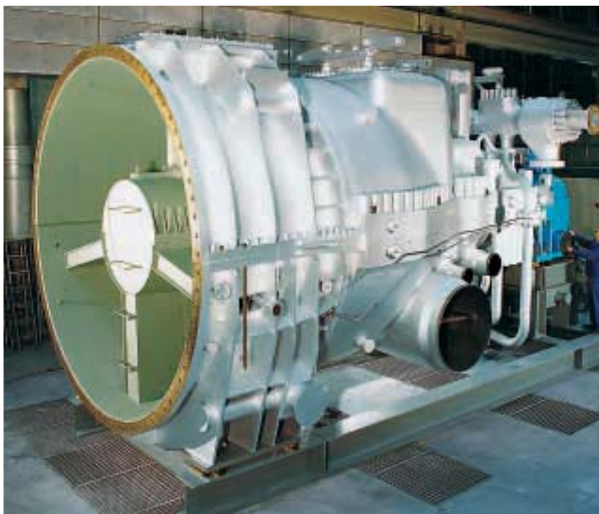
17 Condensing steam turbine with axial exhaust on transport frame
