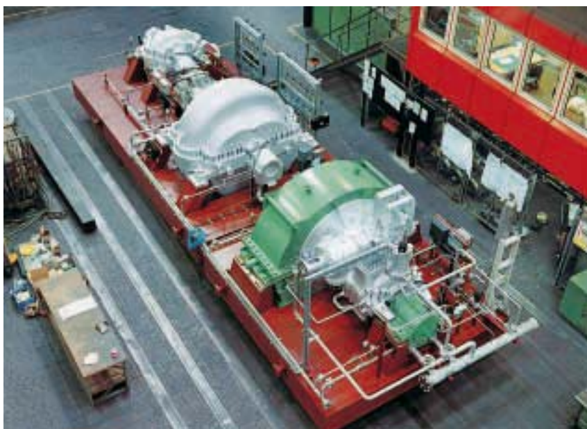
31 Compressor train with condensing steam turbine
