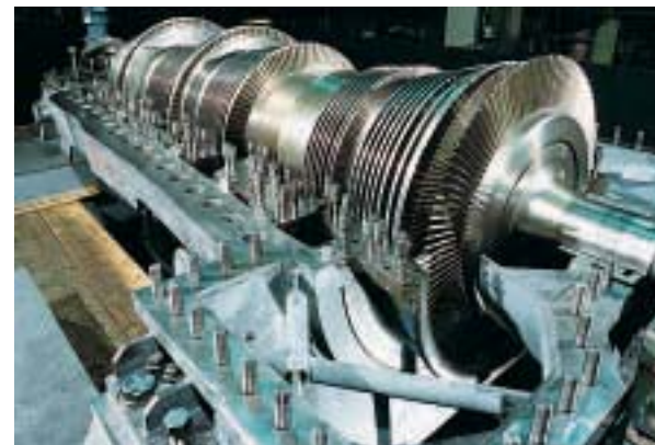
14 25 MW double-extraction condensing steam turbine
