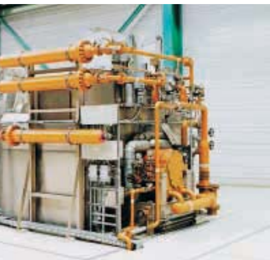
4 Steam turbine generator set
