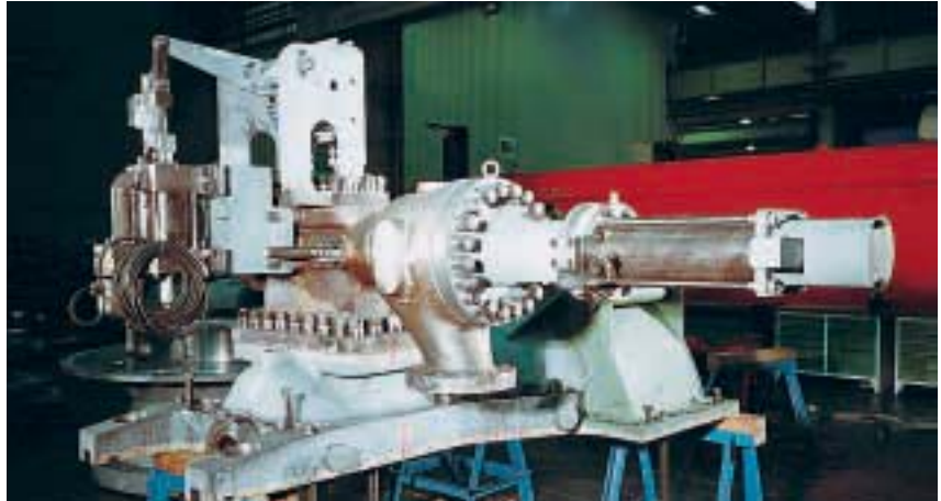
21 Steam turbine upper section with flanged steam chest
